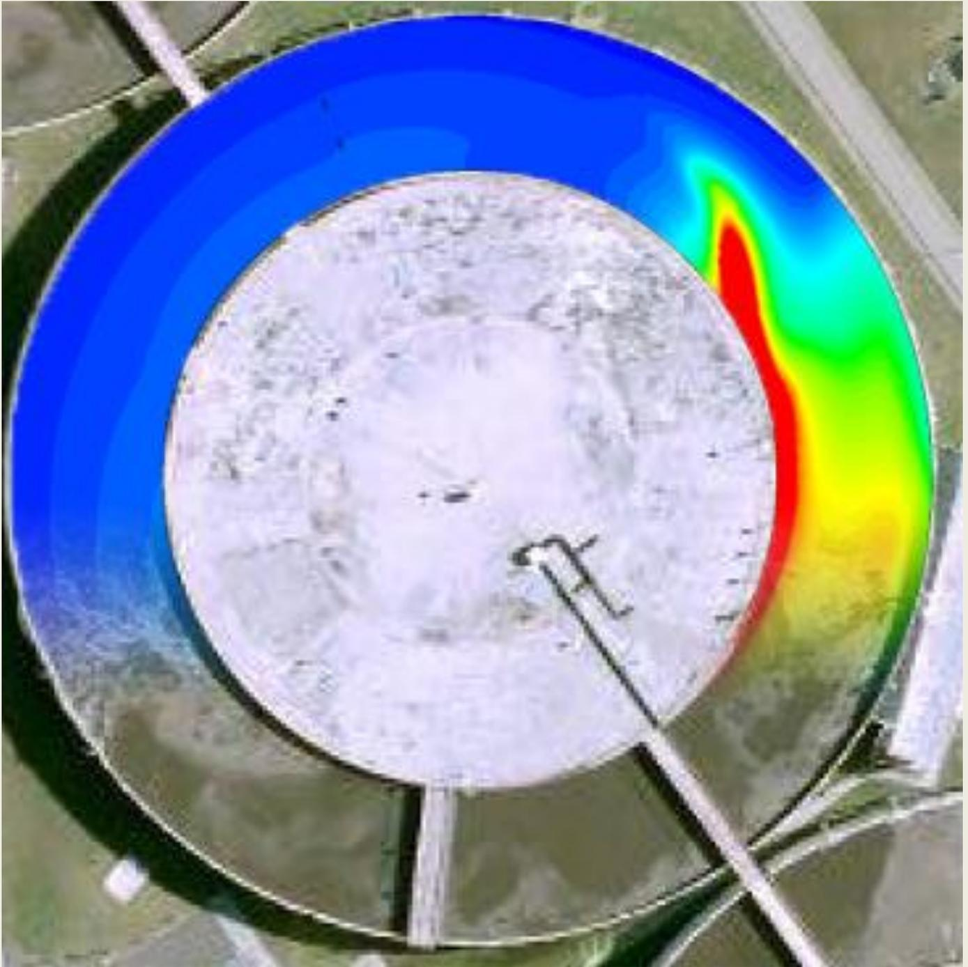
**Next generation bioreactor models for wastewater treatment systems by means of detailed combined modelling of mixing and biokinetics**
