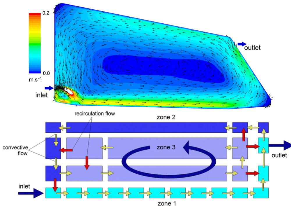
Fig.2 CFD velocity contours and compartmental model configuration
